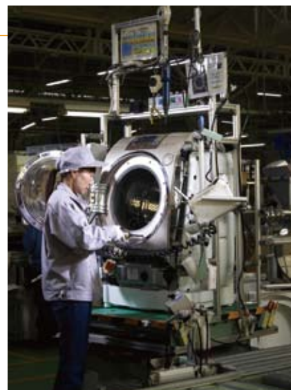
Front loading washer-dryers are assembled in a cell production system.
